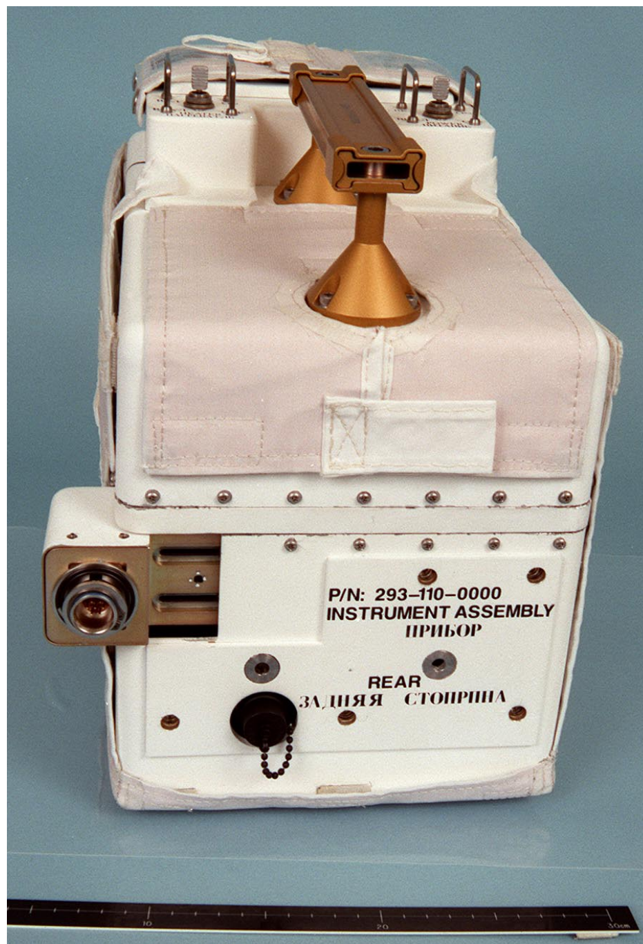
Figure ISS-52 Rear View, without Battery Housing, Battery Electrical Center at Left with the Fuse Cap Underneath
